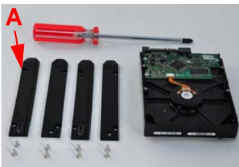
Attach the bracket labeled **TOP** as shown. Point the tapered end towards the hard disk's connection end **(A)**. Use two of the included screws to attach the chassis bracket to the hard disk. Attach the **BOTTOM** bracket to the other side of the hard disk in a similar manner.
