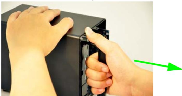
4. Pull the top of the handle up and out to release it.
