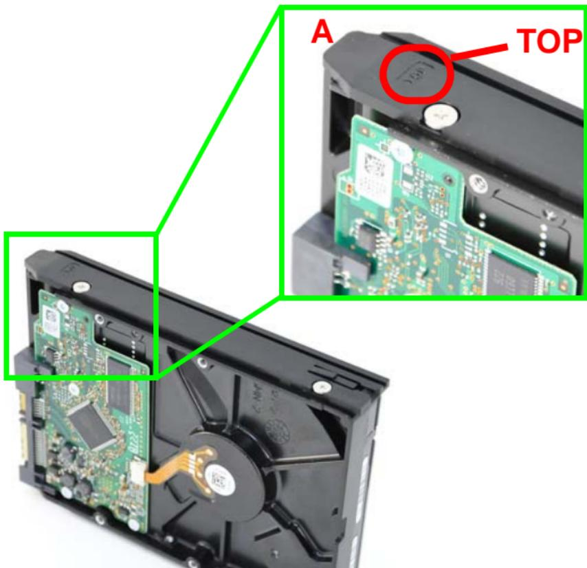
4. Align the hard disk with an NSA bay as shown and slide it all the way into the bay.
