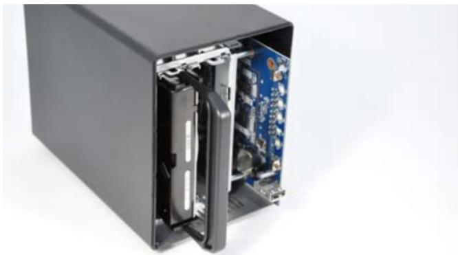
3. Hold the NSA and push your thumb against the front of the chassis and pull the hard disk out.
