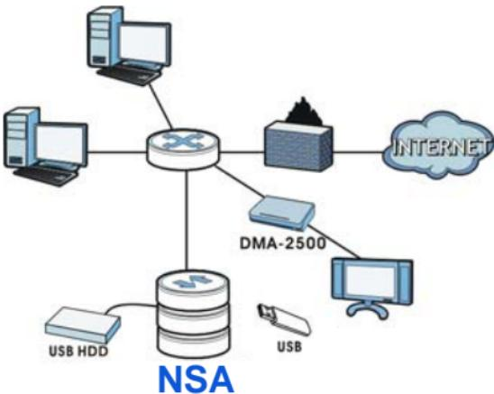
Above is the NSA in a home network. Users back up and share data on the NSA. The DMA-2500 plays the NSA's media files on the TV. A USB hard drive provides extra storage space and files are copied directly from the USB memory stick to the NSA by using the **COPY/ SYNC** button.
