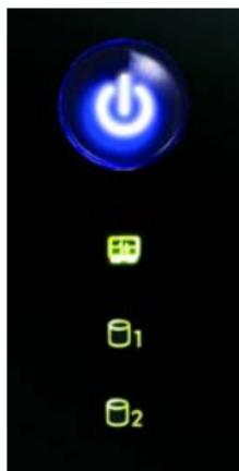
To turn off the NSA, press the power button in and hold it until you hear a beep. Then release the button.
