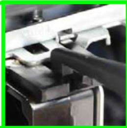
2. Push the other handle end into the notch on the bottom chassis bracket. Make sure the handle is locked into both notches.
