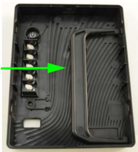
1. Place one end of the handle in the top chassis bracket notch.
