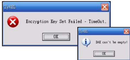
Figure 32 Incorrect DAK or No DAK
