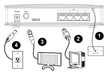
LAN: Use the included Ethernet cable to connect the LAN port to a computer. CATV: Use a coaxial cable to connect the CATV port to a television or set-top box with an F-connector.
