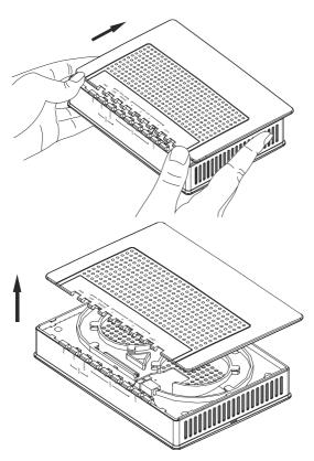
**a.** Hold the ONU-6040BF-2x upright, push the top cover forward with the LEDs (lights) facing you, then lift up the top cover to remove it.
