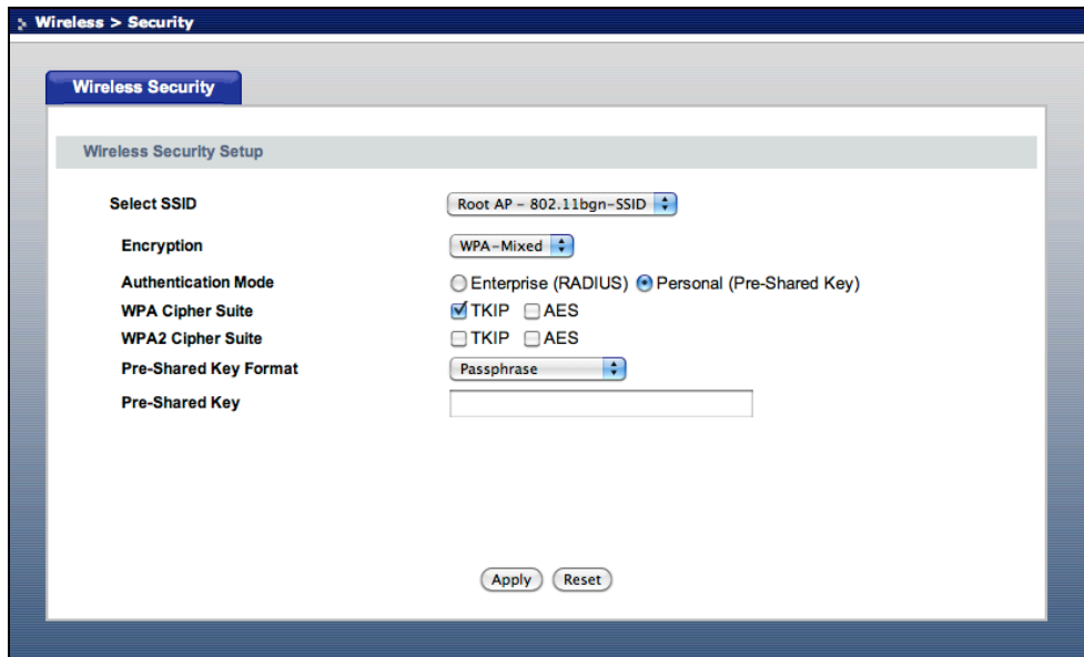
Wireless Security Setup window for WPA-Mixed (Personal (Pre-Shared Key))
