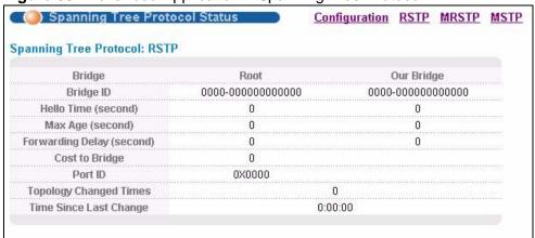
This screen differs depending on which STP mode (RSTP, MRSTP or MSTP) you configure on the Switch. This screen is described in detail in the section that follows the configuration section for each STP mode. Click **Configuration** to activate one of the STP standards on the Switch.
