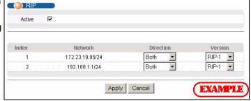
4 Click **Apply** to save your changes back to the run-time memory. Settings in the run-time memory are lost when the Switch's power is turned off.
