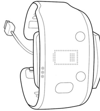
Align the two contacts on the back of your miCoach FIT SMART with the contact points on the charger. With the contacts lined up, your miCoach FIT SMART and the charger should click together.
