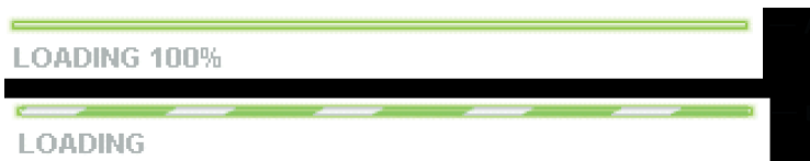
Top. Determinate ProgressBar control Bottom. Indeterminate ProgressBar control
