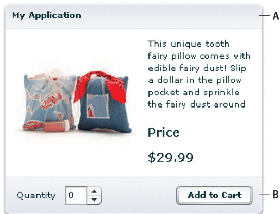
A. Panel container B. ControlBar container
