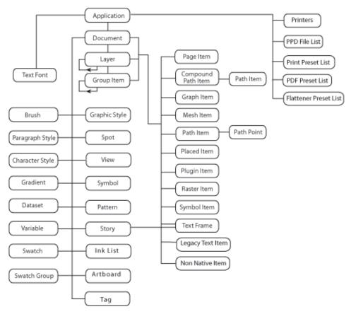
In addition to this application-specific object model, JavaScript provides certain utility objects, such as the File and Folder objects, which give you operating-system-independent access to the file system. For details, see JavaScript Tools Guide.
