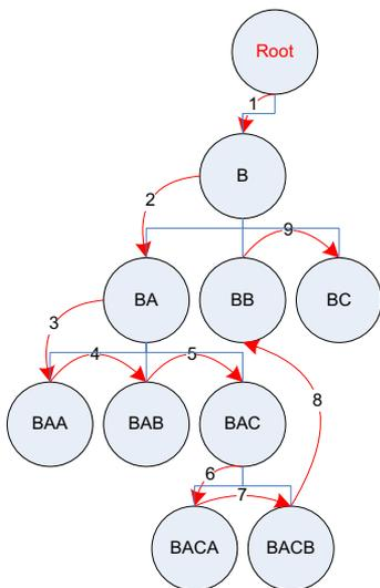
Iteration with `__processChildren` (assuming a rule that matches every XML element in the structure) is shown in the following figure:
