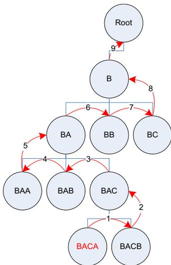
Iteration given the following rule set is shown in the figure after the script fragment. The rule set includes two rules that match every element, including one that uses `__processChildren`. Every element is processed twice. (For the complete script, see `ProcessChildren`.)
