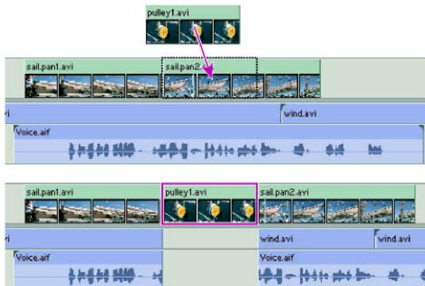
Clips before an insert edit (top) and after an insert edit (bottom)
