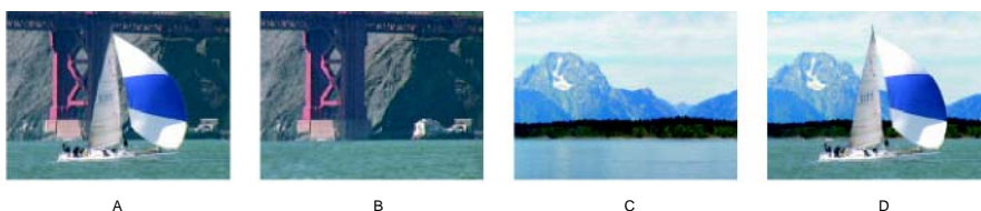
Difference Matte Key A. Original image B. Background image C. Image on second track D. Final composite image
