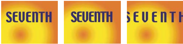
Tracking set to default value of 0 (left), Tracking set to -50 (center), and Tracking set to 200 (right)
