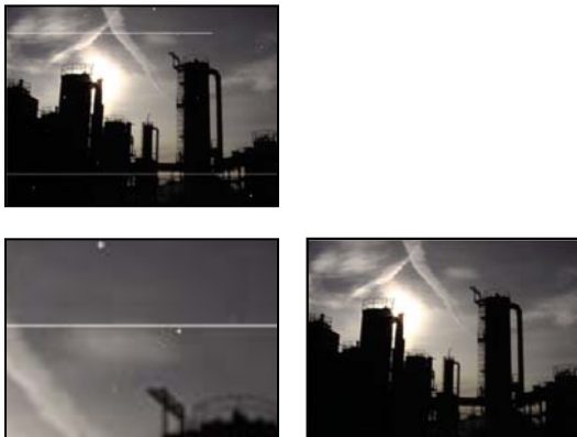
Original image with scratches (upper-left), enlarged view of scratches (lower-left), and scratches removed with loss of clarity (lower-right)
