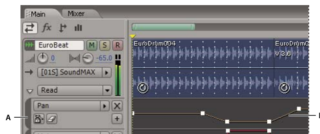
Automating track settings in the Main panel A. Automation lane B. Envelope for parameter
