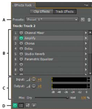
A Rack Preset controls B Effect slots C Level controls D Main Power button
