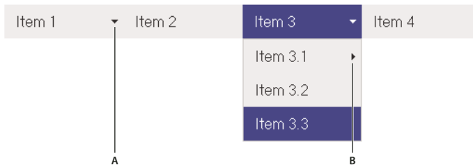
Menu Bar widget (consists of <ul> , <li> , and <a> tags) A. Menu item has submenu B. Submenu item has submenu
