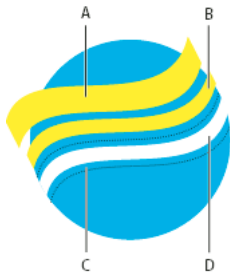
A Overprinted top stroke creates spread trap B Bottom stroke creates knockout C Area of knockout D Area of trap
