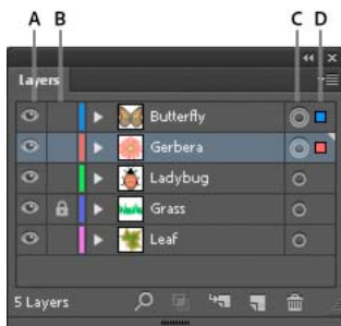
A Visibility column B Edit column C Target column D Selection column
