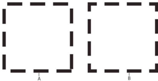
A Preserved exact dash and gap lengths B Aligned dashes to corners and path ends, adjusting lengths to fit
