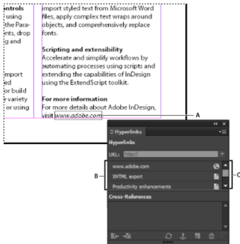
A Hyperlink source B List of hyperlinks in the current document C Hyperlink status icons
