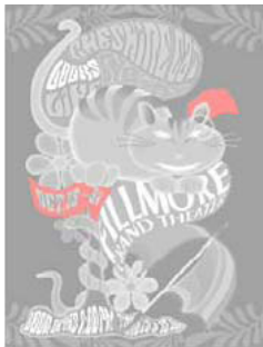
Areas that exceed the specified ink coverage limit are shown in red.
