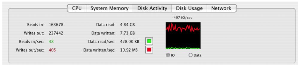
To be certain that you are I/O bound, we need to compare this activity rate with your maximum read/write rates. For each disk, there is a maximum read/write rate (which may be much less than the disk's advertised transfer rate). While it is easy to watch current read/write rates using Activity Monitor, it is harder to determine your maximum read or write rate. Typically, the I/O bottleneck is writing to disk.
