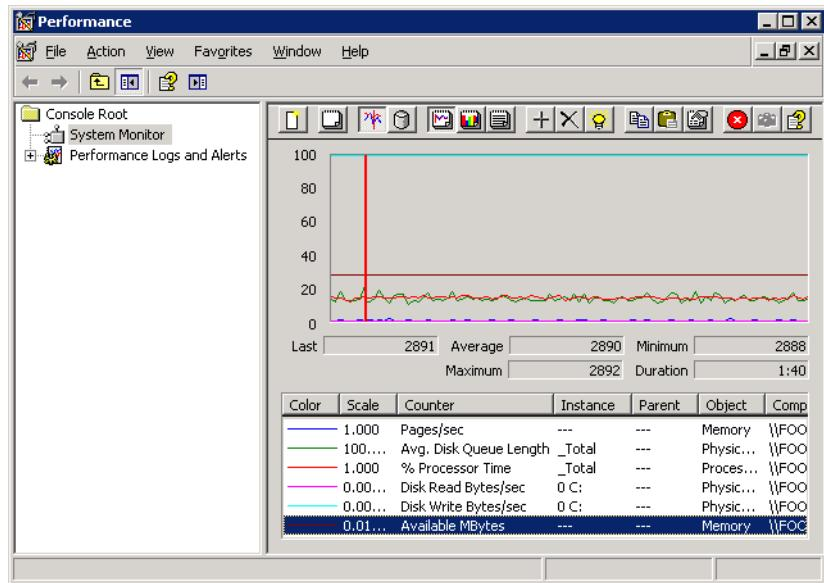
Note in the preceding test how low CPU usage is, as shown by the red line running also at about 20. In a test that exhibits this behavior, a more powerful processor will not enhance scalability. Note also that we are tracking the disk write rate on the light blue line. This is the number of bytes written to the disk per second. The disk-write rate can help you determine whether you are I/O bound in cases when the disk-queue length is not consistently high.
