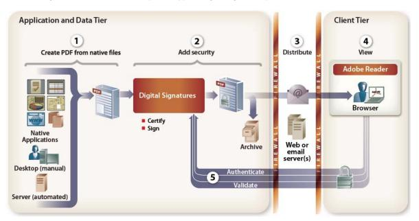
The following illustration shows an example of a typical Digital Signatures process.
