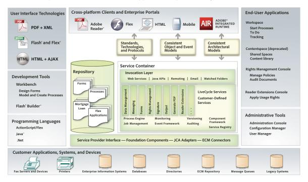
The development area includes Workbench tools and the repository. Development of forms and Guides (deprecated), process flows, and related collateral is done in Workbench. The Eclipse-based development environment can also include Flash Builder (available separately). You can use Flash Builder to develop RIAs, create custom components for use in Guides (deprecated), customize Workspace, and more. (See LiveCycle Workspace Help.)
