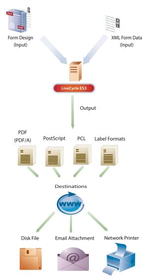
A form author creates the form in Designer. The form conforms to the XML schema that the Output service uses as the XML data input file to create the output.
