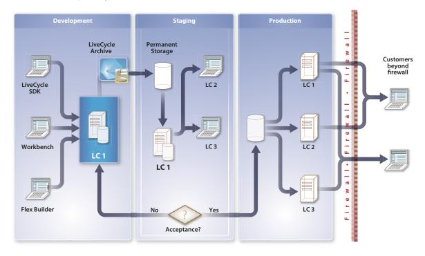
Administrators move all assets (such as PDF forms, images, process diagrams, and other files required) for an application to work from one phase to the next. Developers typically package all application assets into a LiveCycle archive (DSA) file and transfer it from development to staging to production.
