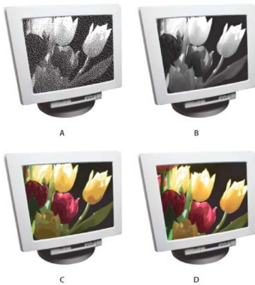
A Bitmap mode B Grayscale mode C Indexed-color mode D RGB mode
