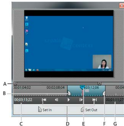
A Zoom control B Clip In point C Current time D Playback controls E Current-time indicator F Clip Out point G Clip duration
