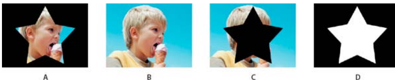
A Clip with alpha channel B Ignore Alpha C Invert Alpha D Mask Only
