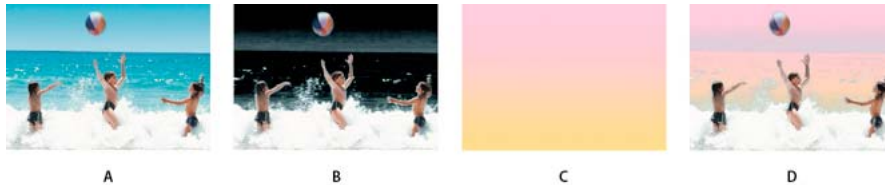
A Original clip B Blue color keyed out C Clip on second track D Final composite clip
