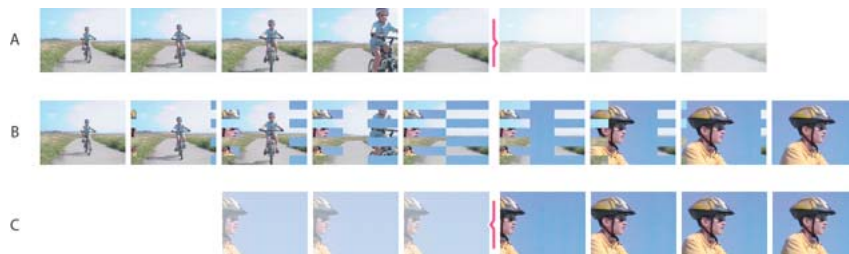
A First clip showing last frame repeated B Movie containing both clips and transition C Second clip showing first frame repeated
