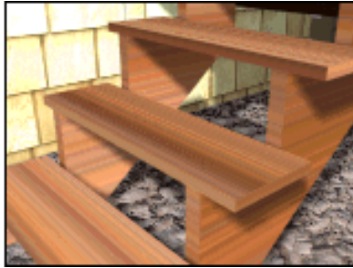
Step depth variance between two stairs
