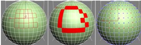
Edge selection (left) converted to face border (center) and vertex border (right)
