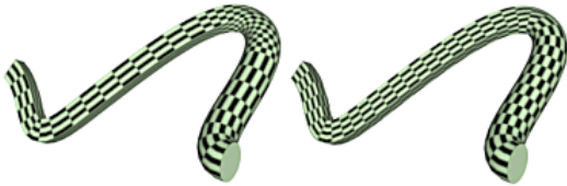
Before and after applying Normalize to loft
