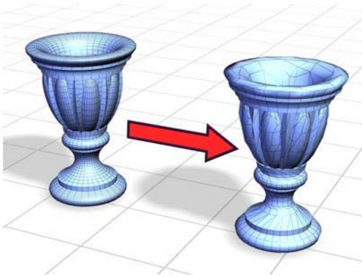
Optimize simplifies a smooth model with a high number of faces without greatly changing the model's appearance.
