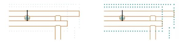
In addition, linetypes with dash and dot combinations display round dots, unlike previous releases that represented dots with very short dashes.
