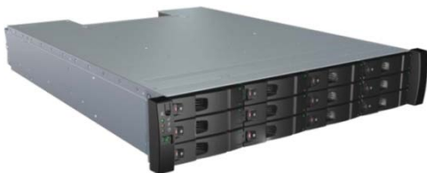
ISIS | 1000 Engine including Storage Controller, 2 power supplies, Media Pack (10 HDDs), and 2 system drives (SSDs)
