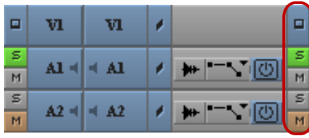
Track Selection panel, with video and audio tracks selected for solo monitoring
