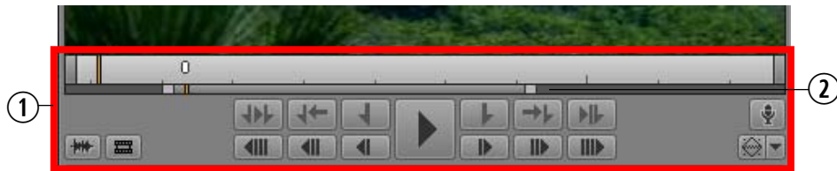
1. Area in which the mouse wheel controls the zoom region. 2. The zoom region within the zoom bar.
