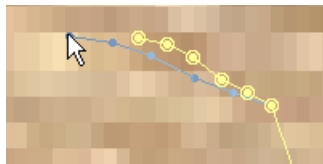
When you stretch by moving one end point, the point at the other end of the range becomes the anchor while you drag the moving point. After the stretching process, all the selected points are relocated proportionally between the point you have dragged and the anchor point.
