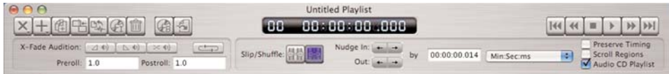
The Playlist's Control Area contains the Playlist Function buttons, Crossfade Audition Controls, Counter display, Nudge Controls, Transport Controls and Mode Checkboxes
