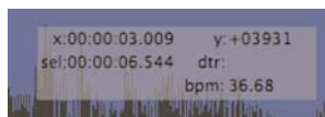
The cursor overlay follows the mouse cursor as it moves, and displays various types of information directly over the waveform
