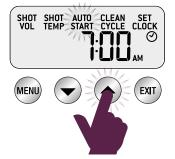
Press UP or DOWN arrow to adjust AUTO START to the desired time. (default AUTO START time set at 7:00am). Press EXIT button. Machine will beep once to confirm setting.
