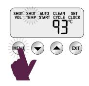
Press UP or DOWN arrow to adjust SHOT TEMP to the desired setting (range  $86^{\circ}$ C -  $96^{\circ}$ C).
