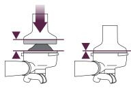
As a guide to dose, the top edge of the metal cap on the tamper should be level with the top of the filter basket AFTER the coffee has been tamped.
