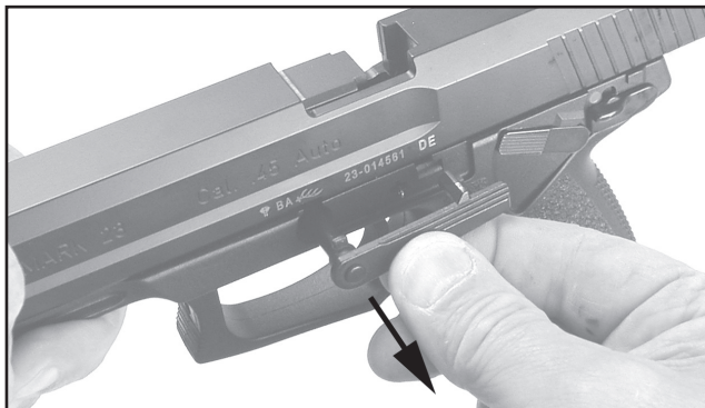
Figure 8 Removing the Slide Release
