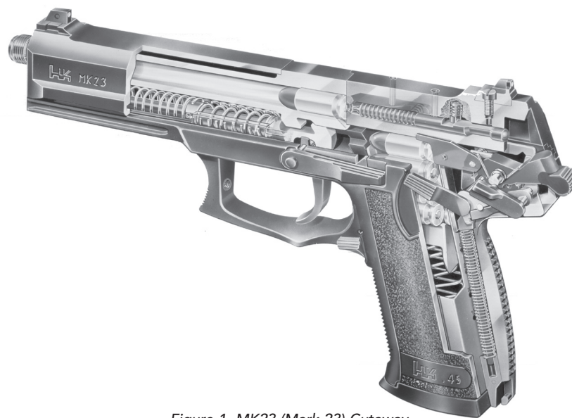
Figure 1 MK23 (Mark 23) Cutaway
