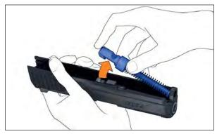
Fig. 41b: Removing recoil spring
