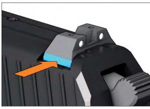
*Fig. 28a: Shifting the rear sight laterally*
