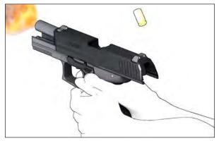
*Fig. 33b:* Path of the slide
