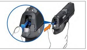
Fig. 25a: Pressing the decocking lever
