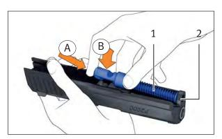
Fig. 43a: Inserting the recoil spring
