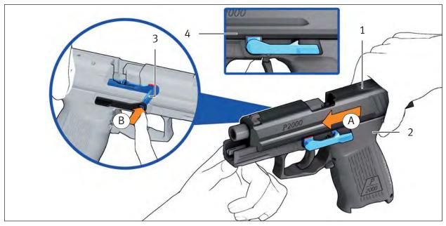
*Fig. 40b: Pressing in slide release axle*
