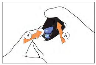
*Fig. 30c: Pushing cartridge to the rear*
