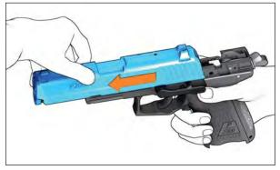
Fig. 41a: Removing slide from frame
