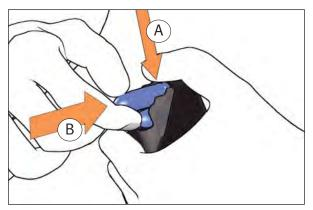
*Fig. 30b:* Pushing cartridge under the magazine lips
