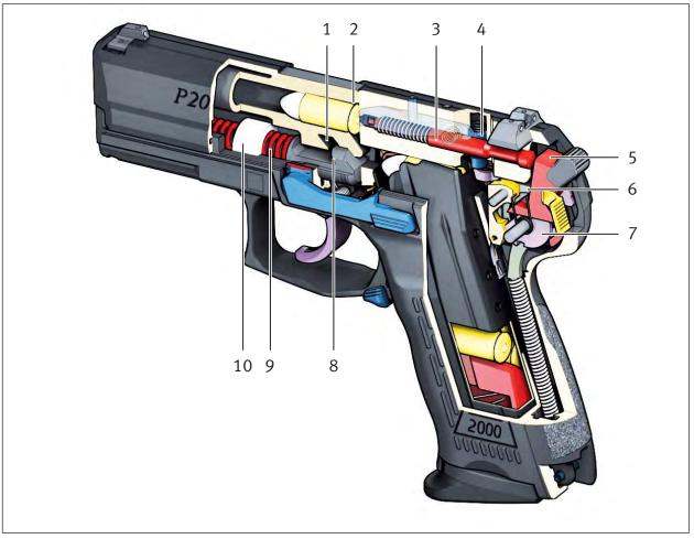
*Fig. 13a:* CDA trigger variant, cutaway view
