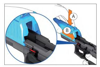
*Fig. 43c: Push the slide onto the frame*
