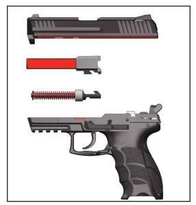
Figure 47 — Lubrications Points (in red)
