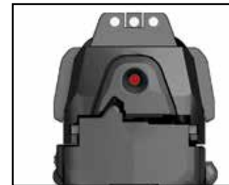
Figure 11 — Firing pin cocked
