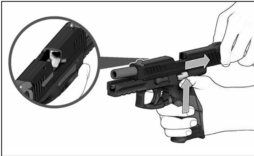
Figure 4 — Clearing the VP Pistol
