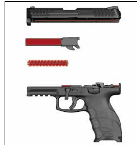
Figure 33 — Lubrication Points (in red)
