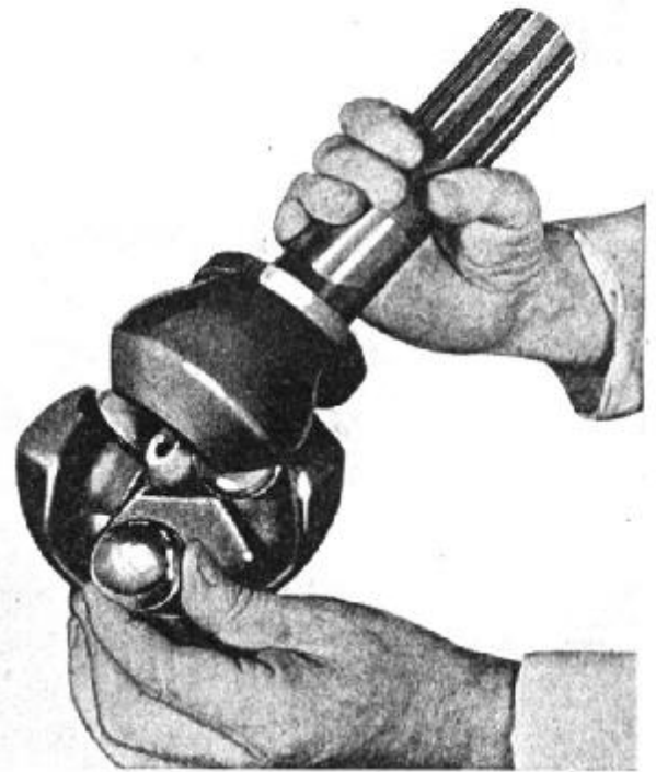
FIG. 7—ASSEMBLING UNIVERSAL JOINT BALLS
