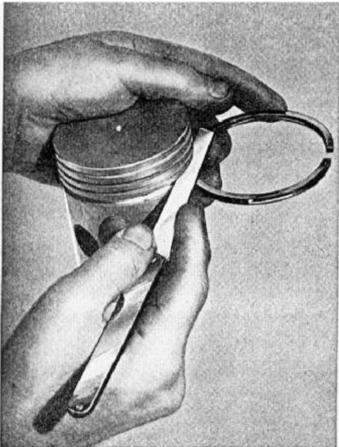
FIG. 27—OIL RING FITTING
