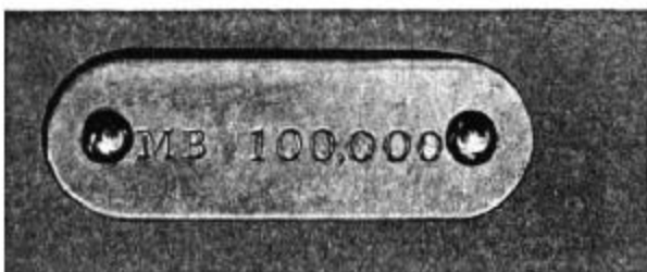
Chassis Serial Number located on inside of frame at left front end.
