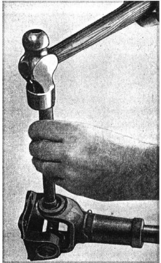
FIG. 3—REMOVING UNIVERSAL JOINT BEARING
