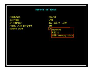
By default the save location for the screen shot will be the USB memory stick; this can be changed in the 'Remote' menu. You can change it to print to the RS232 port, that is used to print to an attached printer to print a physical copy of what is shown on the screen described in 6.4.
