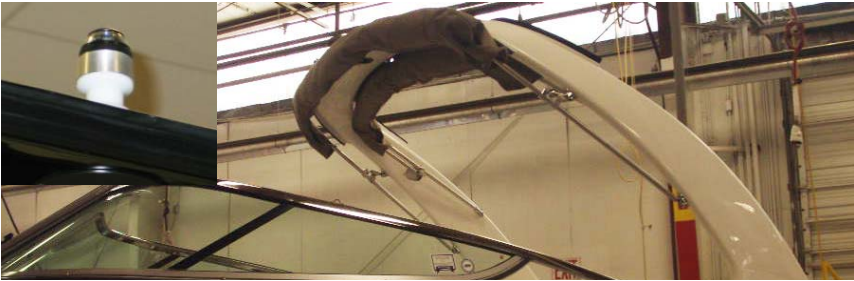
Tower Shown In Up Position
