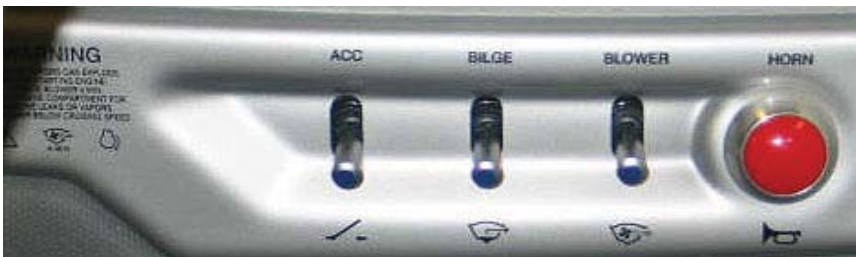
Typical Starboard Switch Panel
