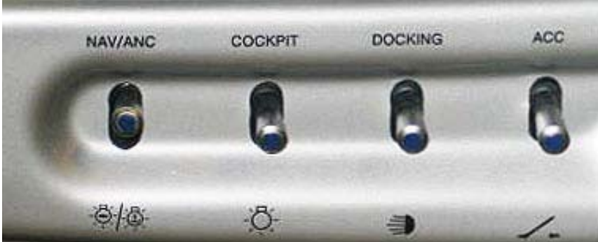
Typical Port Switch Panel
