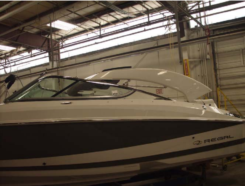
Tower Shown In Forward Tilted Position
