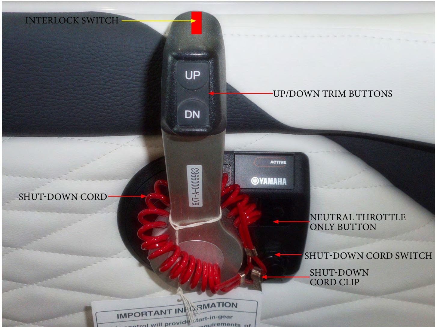
TYPICAL DIGITAL CONTROL SHOWN IN NEUTRAL POSITION
