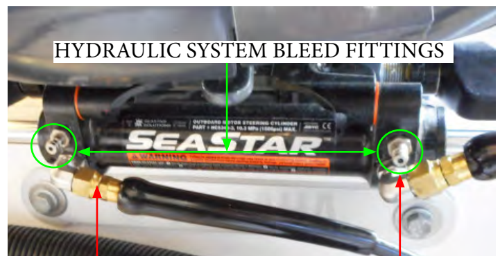
STEERING HARDWARE & HOSES AT ENGINE
