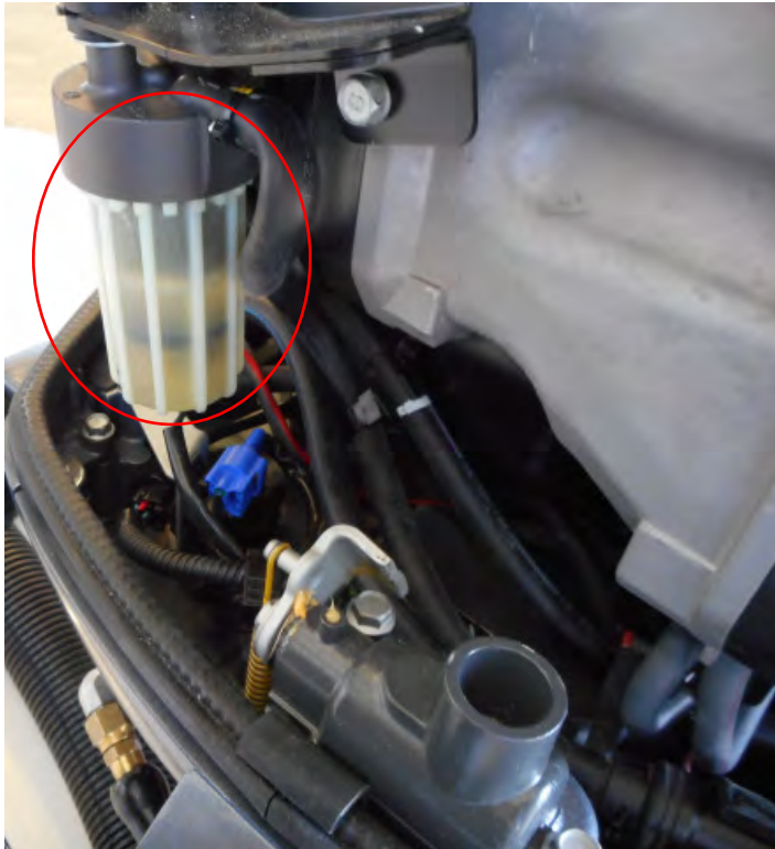
CHECKING ENGINE MOUNTED FUEL FILTER
