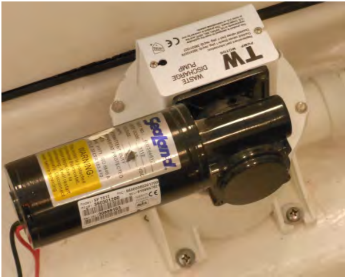
TYPICAL OVERBOARD DISCHARGE PUMP
