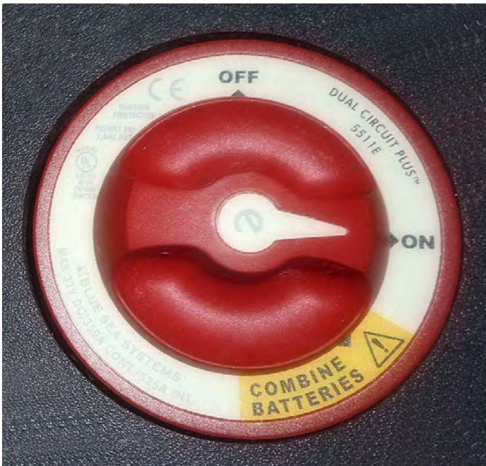
TYPICAL DUAL BATTERY SWITCH
