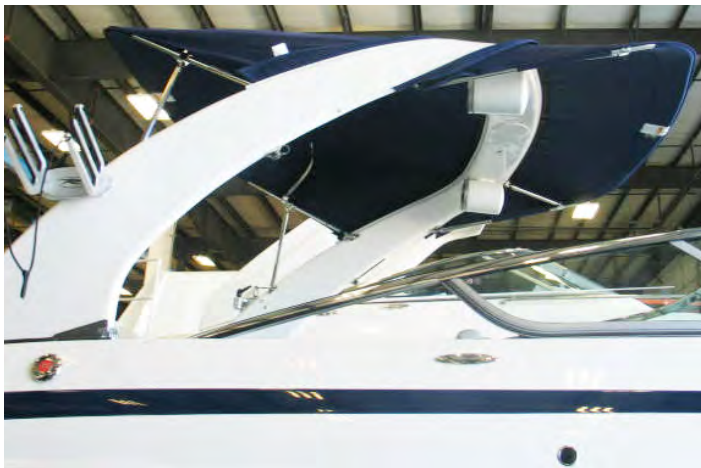
TYPICAL POWER TOWER- SUNSHADES IN CRUISE POSITION
