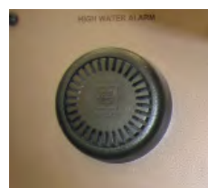
Helm High Water Alarm
