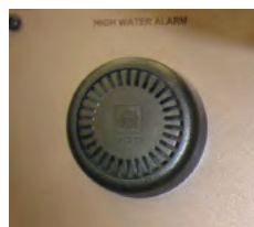
Helm High Water Alarm
