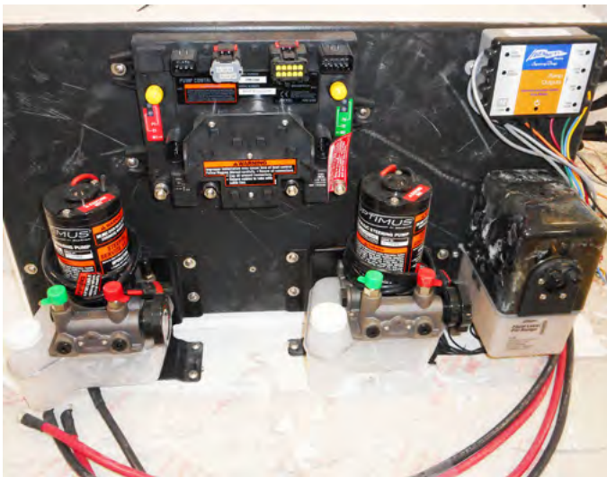
TYPICAL POWER STEERING BOARD
