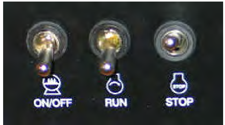
TYPICAL GEN-SET SWITCH CLUSTER- MAIN PANEL
