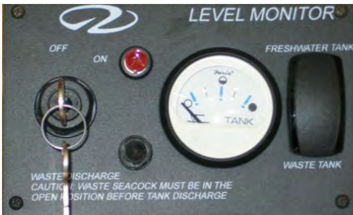
TYPICAL WATER/WASTE MONITOR PANEL
