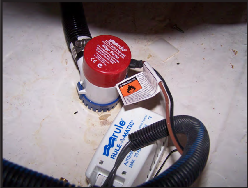
Typical Bilge Pump And Automatic Float Switch
