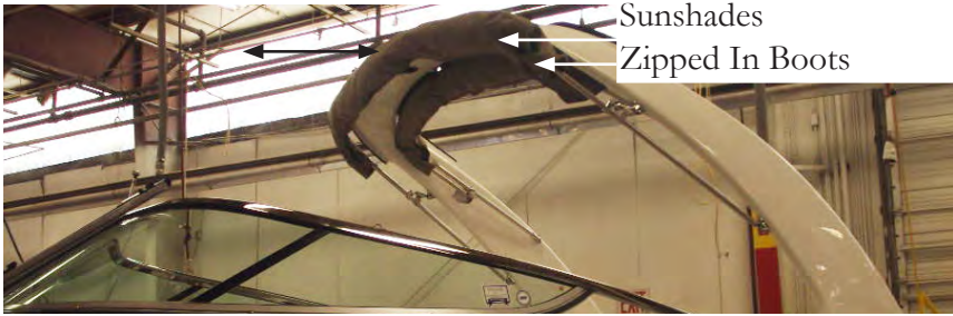
Typical Power Tower Shown In Booted Cruise Position
