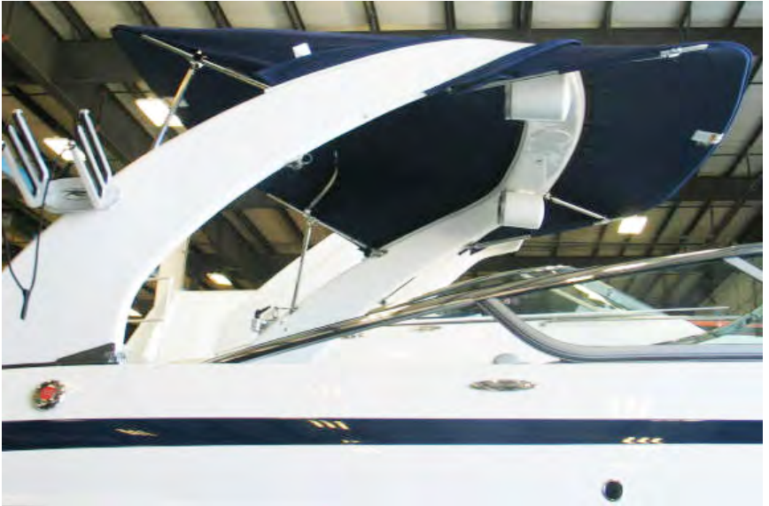
Typical Power Tower- Sunshades In Cruise Position
