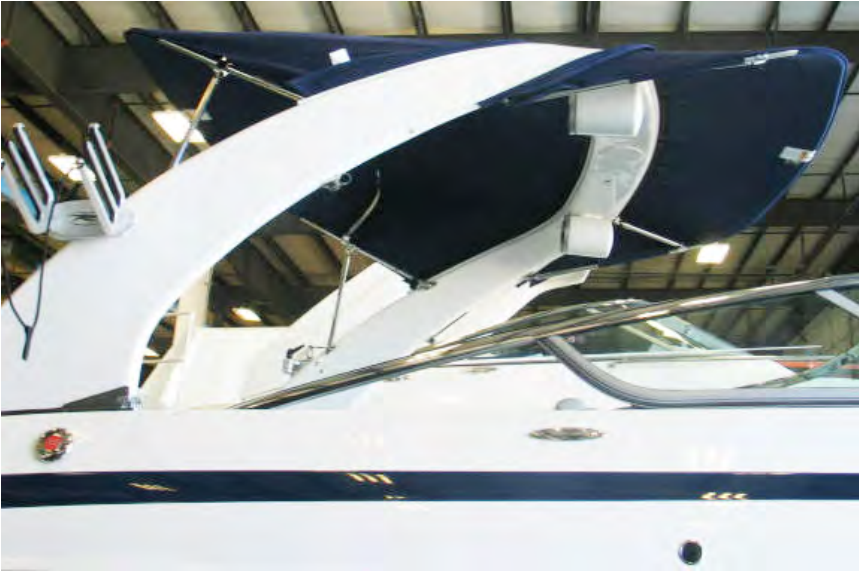
Typical PowerTower In “Up Position w/Sunshades
