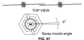
Remove the two ReadySpace spray nozzles and soak the tips in an acetic acid solution (Figure 58).
