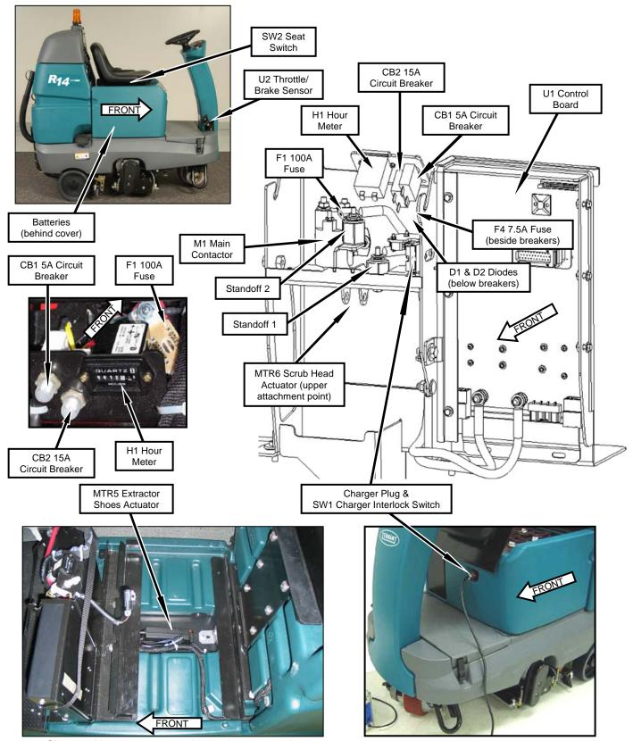
Shown with seat, cover, and batteries removed
