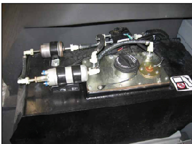
Fuel Pump and Manifold (mounted on fuel tank)
