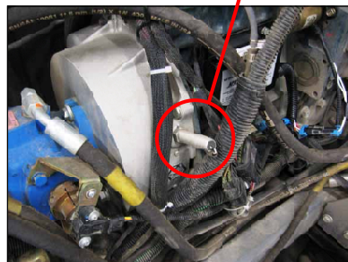
Governor Engine Speed Magnetic Pickup
