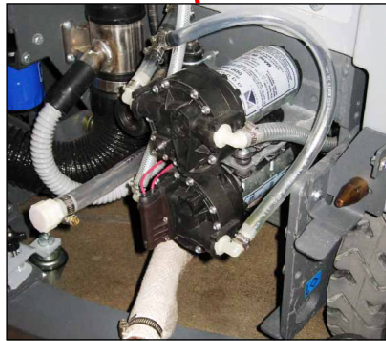
Solution Pump (top) and Wash Pump (bottom)
