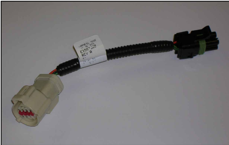
– 56109083 PSI diagnostics cable, 4-pin – 8-pin (Gen1 old style) (see photo)
