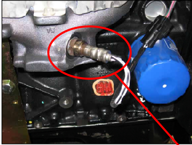
O 2 Sensor (in exhaust manifold) (pre CATCON)
