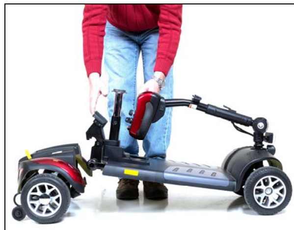
Figure 17. Separating the Drivetrain and Frame
