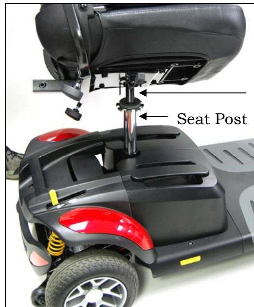
Figure 23. Installing the Seat
