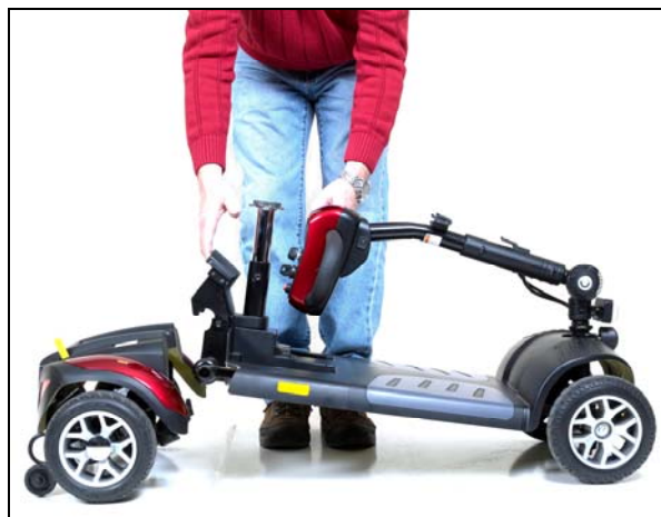
Figure 17. Separating the Drivetrain and Frame
