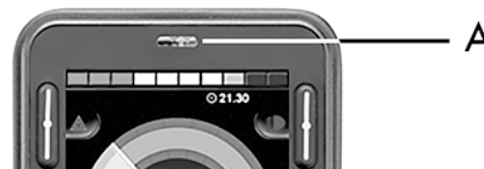
Figure 57. The IR receiver location.
