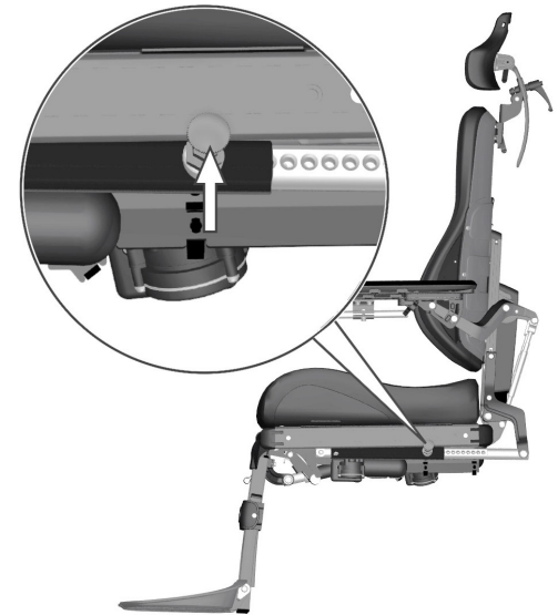
Figure 9. Manually adjusting backrest angle.
