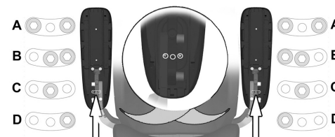
Figure 134. Adjusting the armrest swivel end position.
