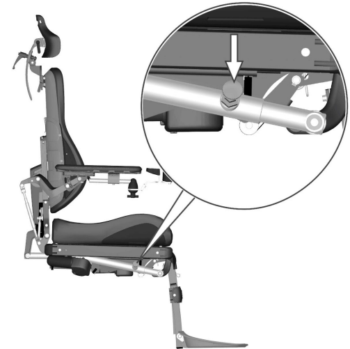
Figure 10. Manually adjusting leg rest angle.
