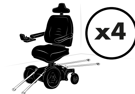
Figure 171. The wheelchair has four tie-down points. The wheelchair and tie-down position in this picture is generic.
