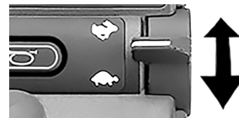
Figure 53. In mode Bluetooth® the right paddle switch is used to scroll up or down.
