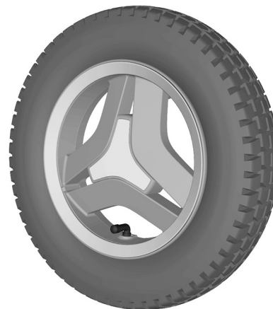
Figure 210. Filling valve on drive wheel.
