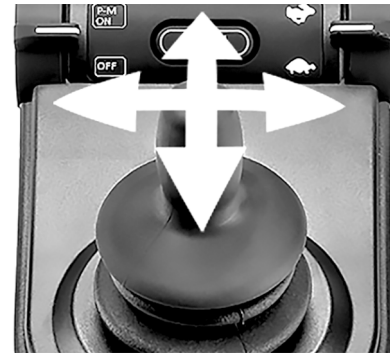
Figure 54. With the use of Bluetooth® the joystick can take control of the mouse functions.
