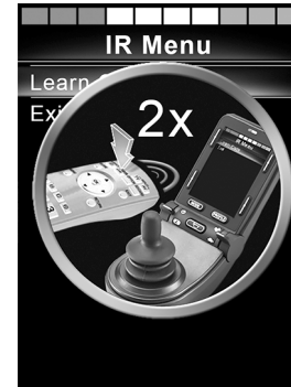
Figure 61 . Point the remote control at the IR receiver. Press the button twice.
