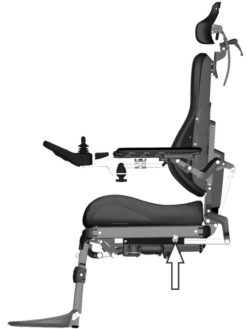
Figure 8. Manual clamp tube for the backrest recline.
