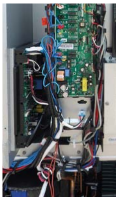
► Comp Wire fix by Holder Wire.
