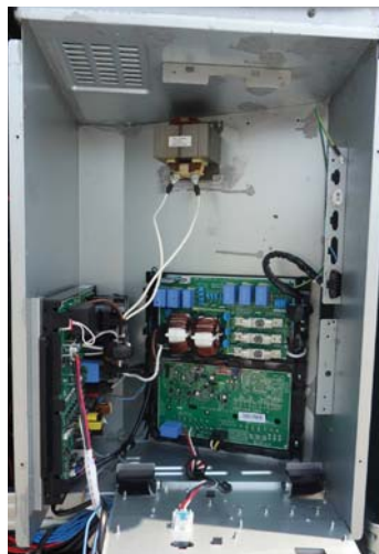
► Separate double layer structure of C/Box after remove 3 screws and connector.
