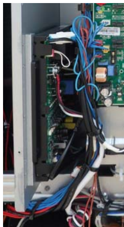
► Comp Wire fix by Holder Wire.
